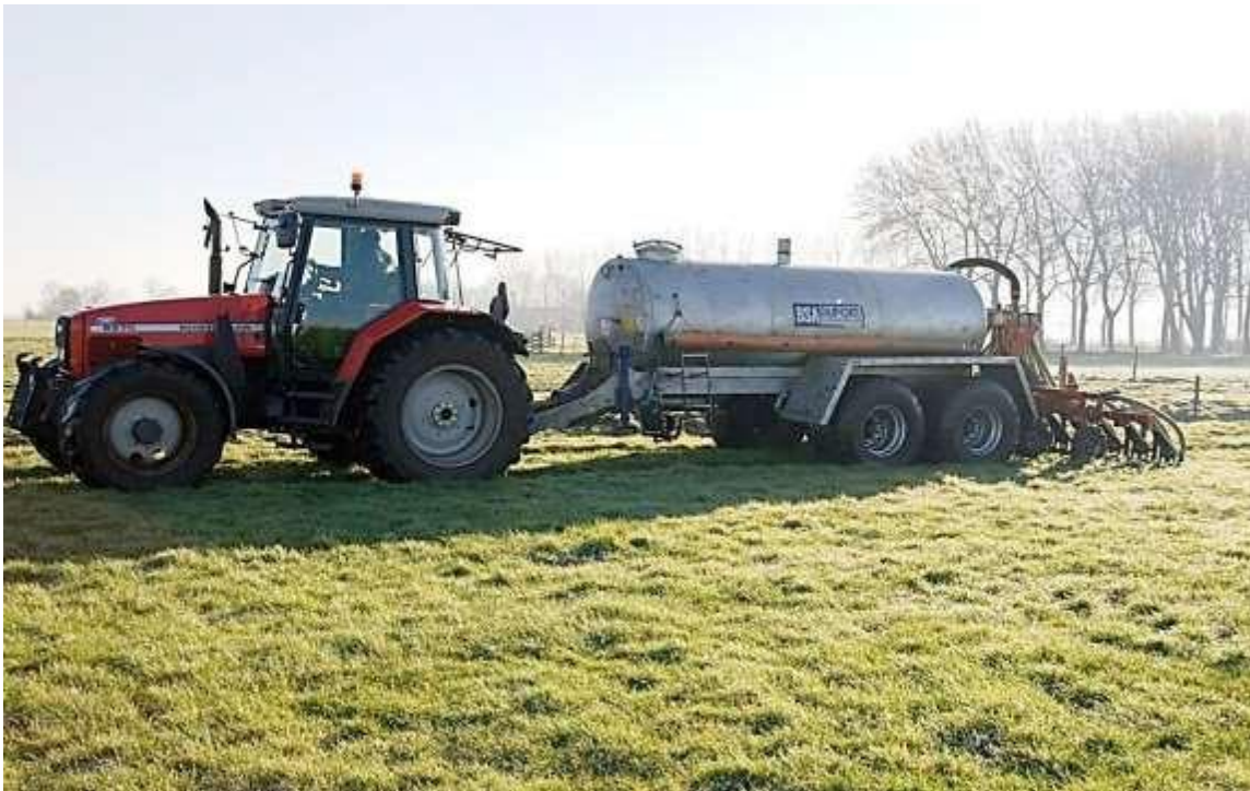
Figure 17: Tanker fed sub-soil injection system
