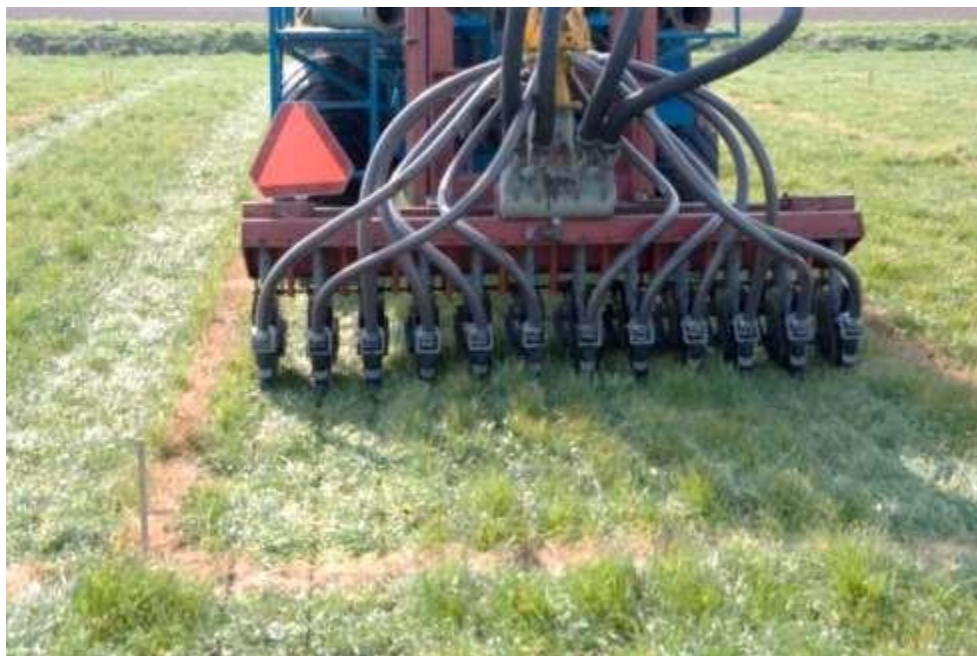
Figure 13: View of injector system mounted on the tanker rear
