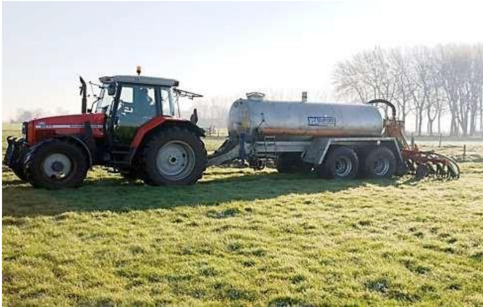
Figure 12: Tanker fed sub-soil injection system
