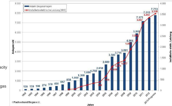
Graph: Number and installed electricity generation capacity (MW) of biogas plants in Germany
