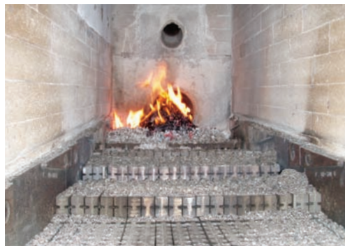
Moving grate from the Fogarty Industries FT-185 Wood Chip Boiler
