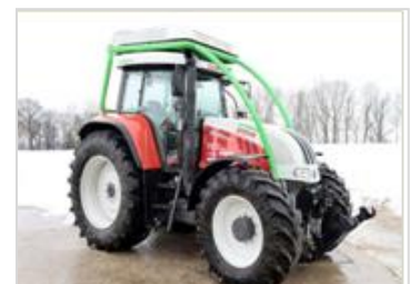
A 200hp tractor running on biomethane, stored in cylinders above the cab (photo courtesy of Biogas plant Margarethen am Moos, Austria).
