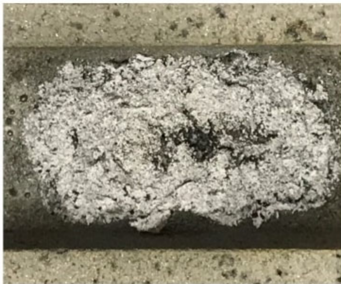
Figure 12. EAF slag reduction using coke
