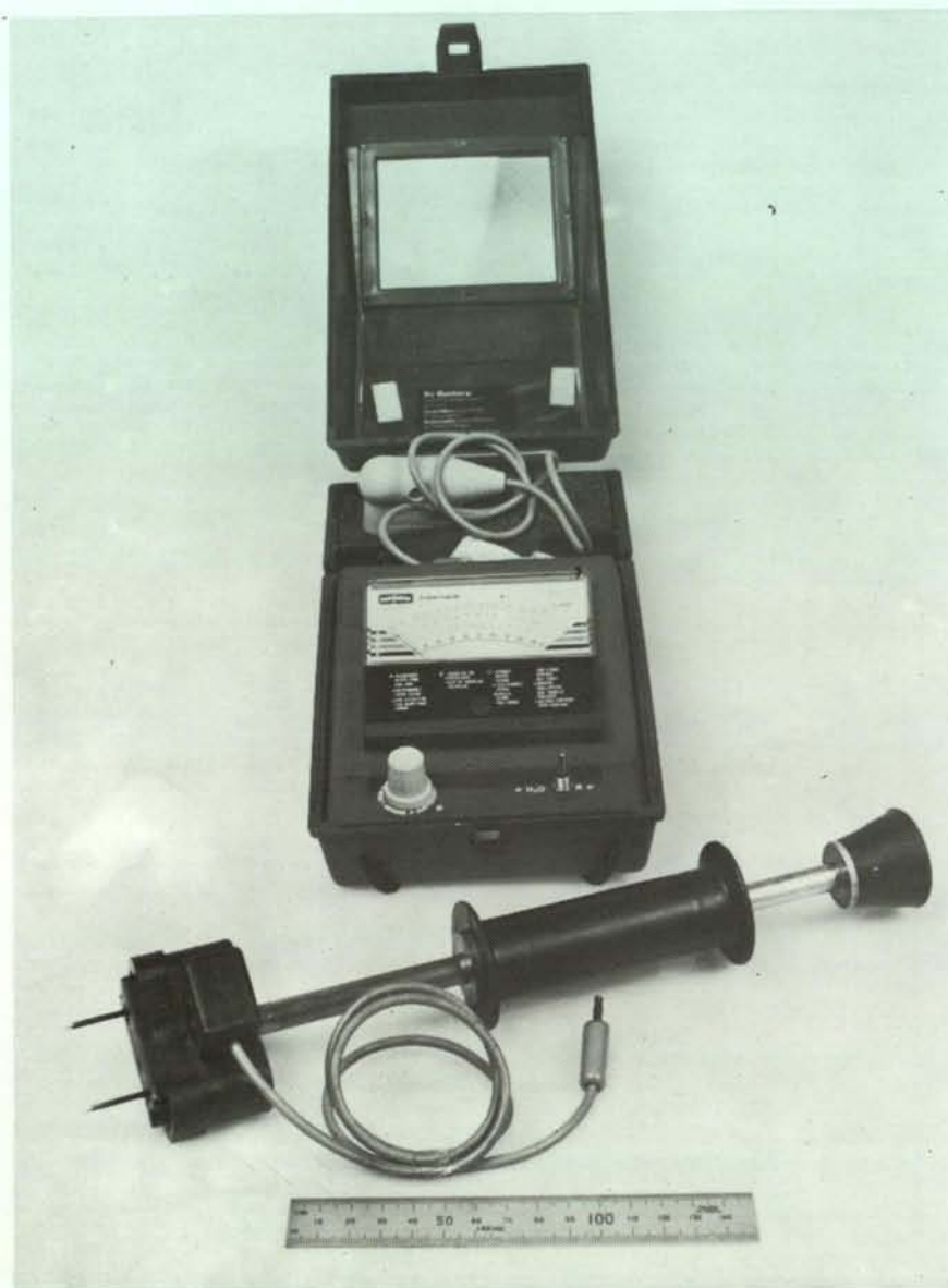
Plate 3. Electric resistance moisture meter with a 'sliding hammer' electrode. Made in the UK.
