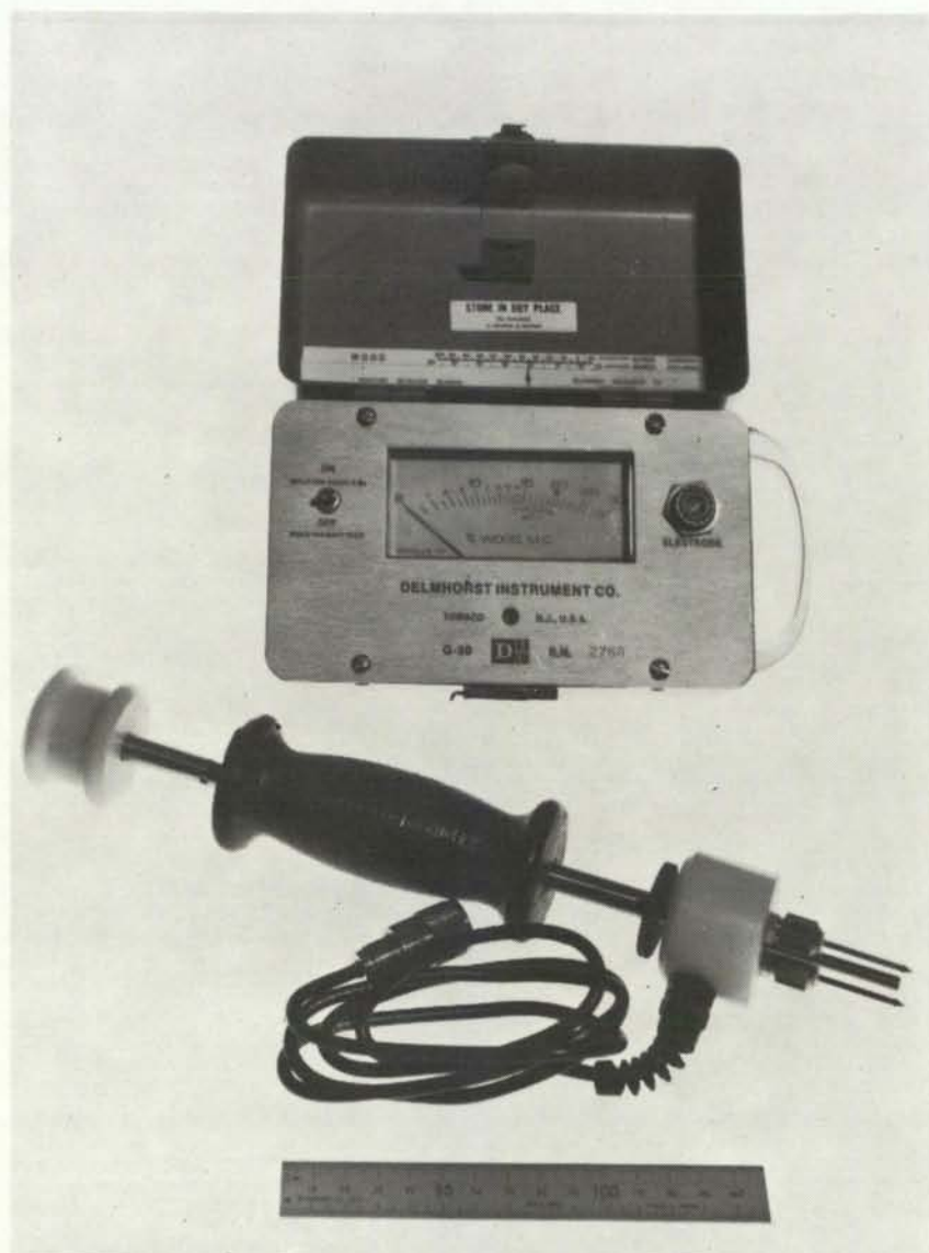
Plate 2. Electric resistance moisture meter with a 'sliding hammer' electrode. Made in the USA.
