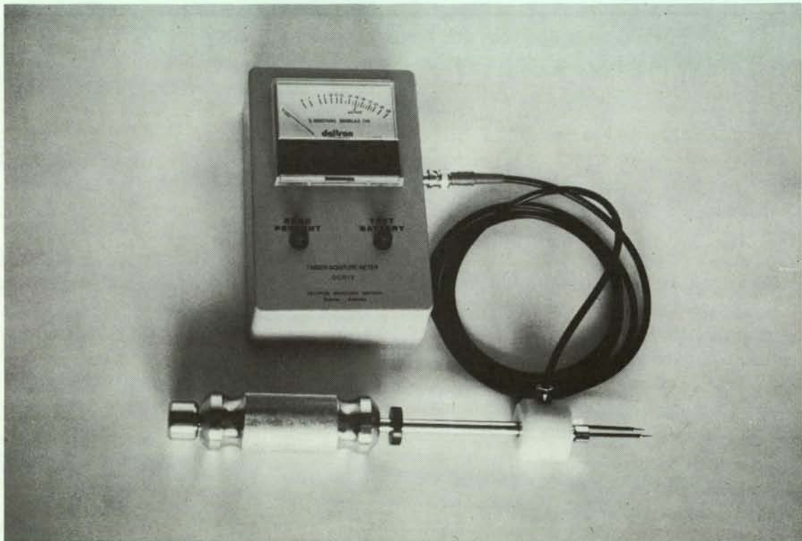
Plate 1. Electric resistance moisture meter with a 'sliding hammer' electrode. Made in Australia.
