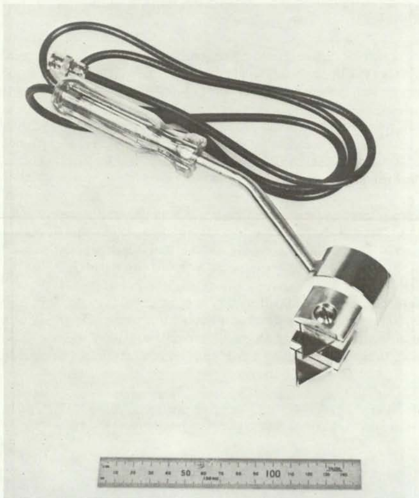
Plate 5. Blade (hammer) electrode for electric resistance moisture meters.
