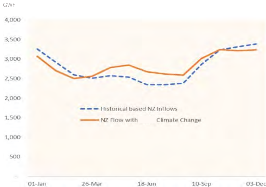
Figure 16: Impact of climate change on average hydro inflows by four week period (modelling completed for NZ Battery project)
